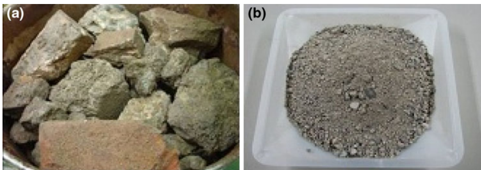
Fig. 1 a Concrete debris in a 200 L radioactive drum, b concrete particles ground up by a crusher
